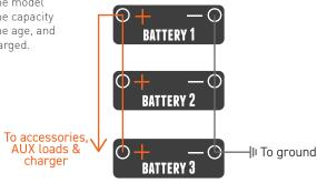
The recommended wiring for connecting multiple batteries in parallel to the BatteryPlus35-II is above. Depending on system requirements, a qualified autoelectrician may wire the batteries differently.
