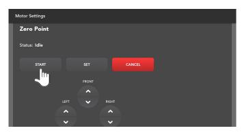
This puts the leveler into zero calibration mode. If active, a status message will display "Calibration Active".
