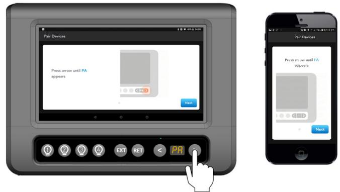
13. When 'PA' appears on the display, press the **EXT** button to start the pairing process to the Node. 'PA' will blink for a maximum of 30 seconds or until a device is connected.
