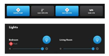
An orange fault indicator will appear on the gas water heater button if a fault is detected on the gas water heater output.
