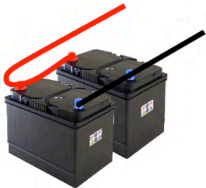
Figure 4: Recommended wiring for connecting batteries in parallel.
